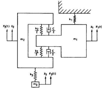
**Figure 2** The three-DOF model representing the rotor bearing set up
