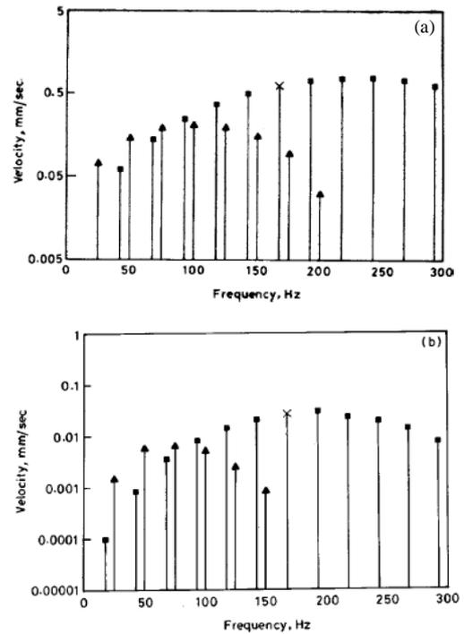
**Figure 3** Frequency spectra for the velocity of the housing for (a) local and (b) distributed defects
