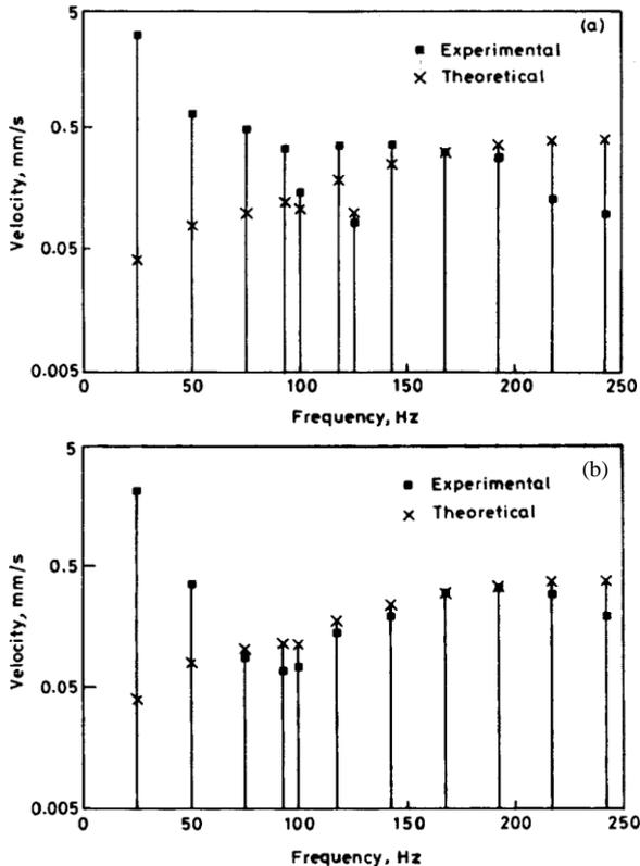
**Figure 4.** Comparison of theoretical and experimental values of amplitudes of spectral components for an NJ 204 bearing at 75 kg load and 1500 rpm with (a) 0.5 mm and (b) 2 mm defect on the inner race
