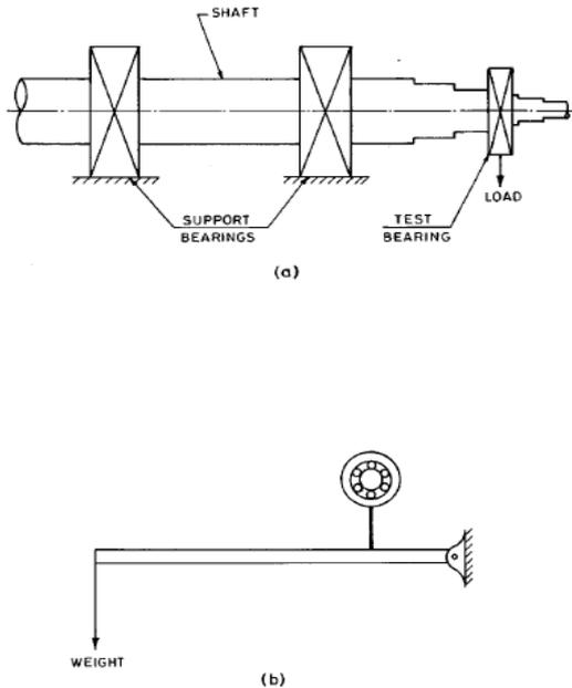
**Figure 1.** A schematic diagram of (a) the rotor bearing system; and (b) the loading arrangement
